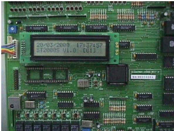
User Interface through Keypad & LCD
